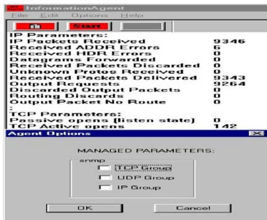
It orients user to make solutions for active network management based on user preferences. There are three groups of parameters that he can actively influence: TCP, UPD, and IP. He can interact and involve its constraints using his proper choice. By means of ISCA control window the user can chose one of three groups of alternatives: TCP, UPD, or IP. The parameters, which are under consid-
