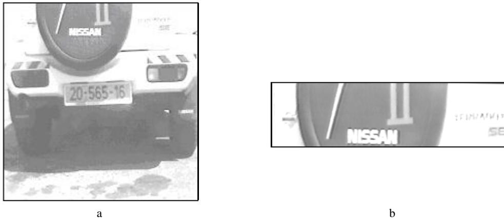
Fig. 5. A source image (a); wrong plate candidate with dominating dark intensity levels, rejected by the gray-level consistency test (b)
