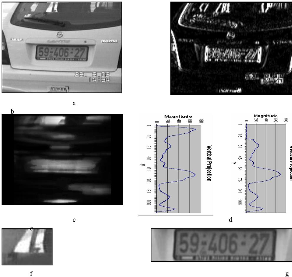
Fig. 6. Illustration of the iterative LPL scheme: image from [2] of original size of  $320 \times 240$  undersampled to  $160 \times 120$  (a); its vertical edge image (b); image after the preprocessing (c); vertical projection of (c) (d); same after zeroing the strip of the rejected plate candidate from (f) (e); proper license plate found at the second iteration (g)
