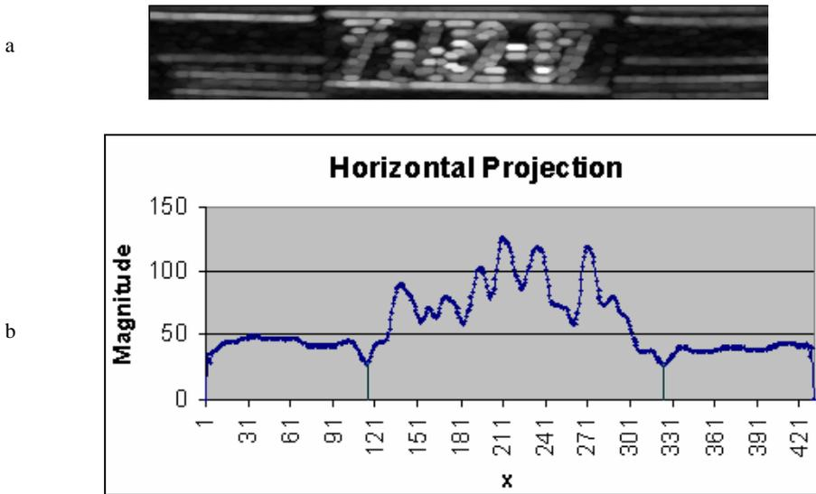
Fig. 4. Horizontal segmentation and plate zone refinement: edge image after erosion operations (a); horizontal projection of (a) with left and right boundaries designated (b).
