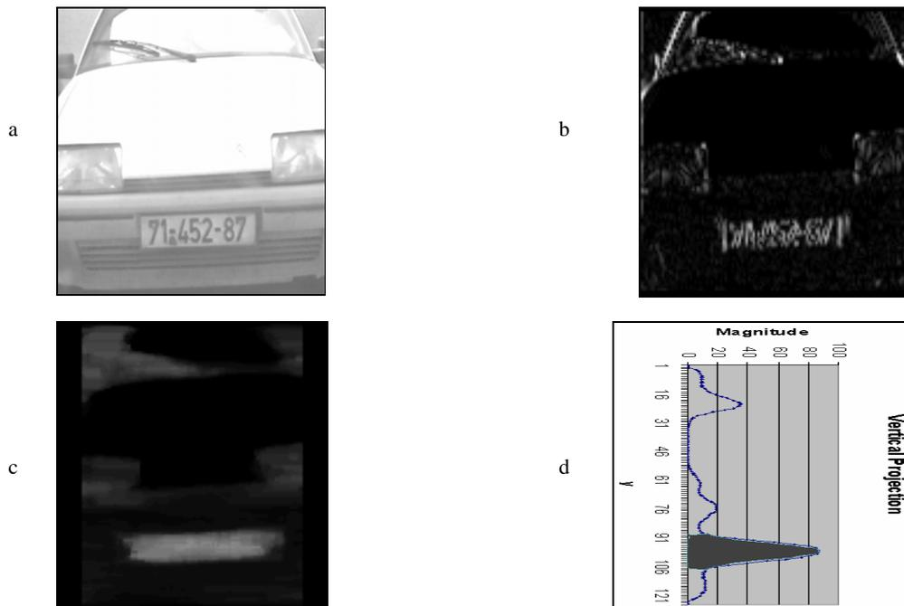
Fig. 2. Original image of 467?500 pixels condensed to a size of 117?125 pixels (a); stressed vertical edge image (b); rank-filtered image (c); vertical projection with the plate strip shown in dark gray (d)
