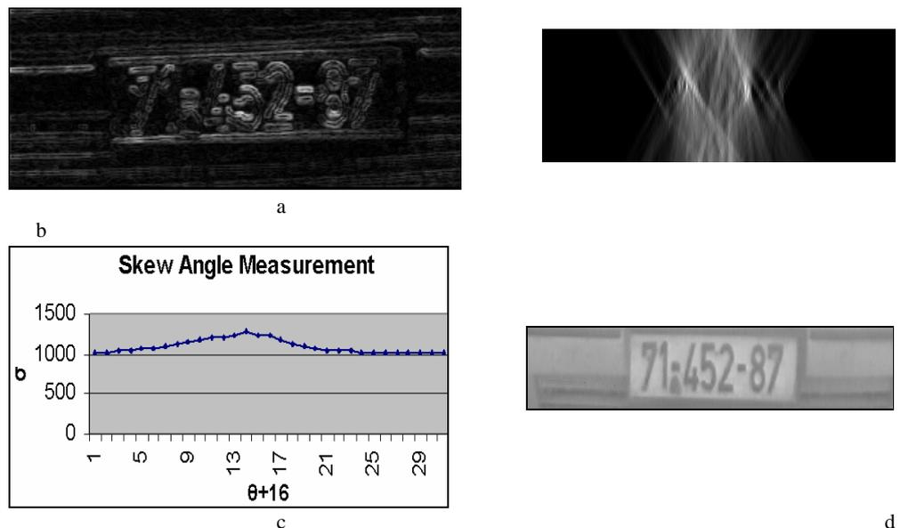
Fig. 3. Skew detection and deskewing: extended image strip with horizontal edges emphasized (a); Radon transform space of (a),  $\theta$  is a vertical axis (b); dependency of  $\sigma$  versus  $\theta$  (is shown in positive range of angles) (c); deskewed image strip of original resolution (skew of  $-3^{\circ}$  was detected, i.e.  $\theta = 13^{\circ}$  on the graph) (d)
