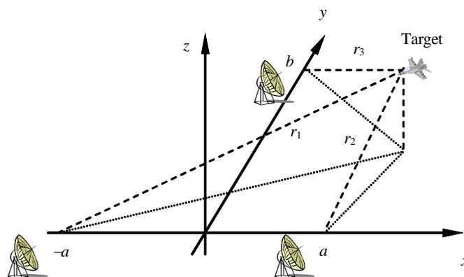
Fig. 1. Diagram of a three-positioned radar system
