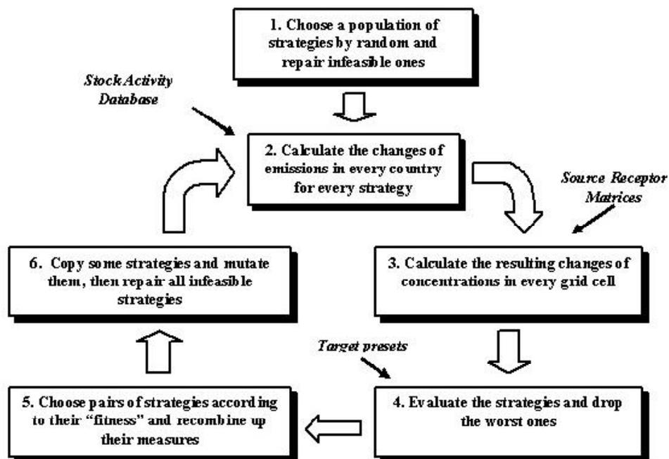
Fig. 3. Implementation of an evolutionary algorithm in IAM
